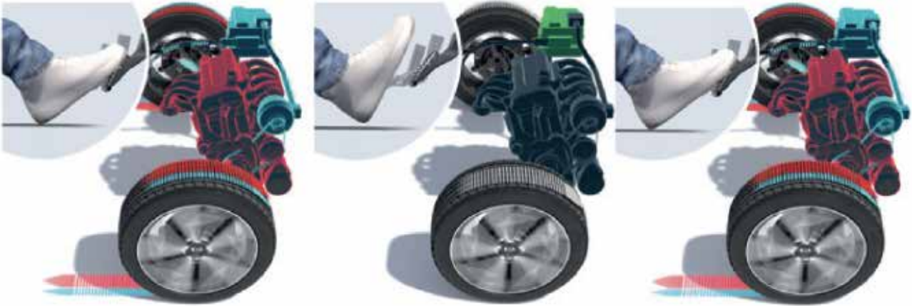
Simplified visual representation of the Mild Hybrid iMT sailing operation.
